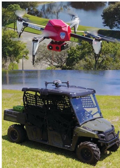
Tethered drones offer unlimited flight times because they receive continuous power through the tether, and they are generally safer because they’re not free-flying, which makes them easier to train security officers to successfully launch and operate. Photo courtesy of Hoverfly
